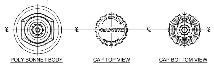
3. PLACE BONNET CAP OVER BONNET BODY AND PRESS ON OVER FIRST SNAP ONLY. (SECOND SNAP LOCKS THE CAP IN PLACE)
