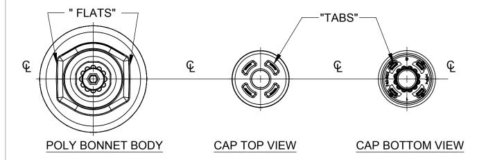
2. PLACE BONNET CAP OVER BONNET BODY AND PRESS ON OVER BOTH SNAPS. CAP SHOULD NOT BE EASILY REMOVED FROM BONNET AFTER ASSEMBLY
